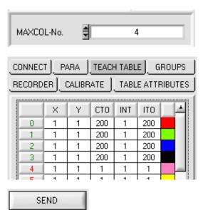
In this example, MAXCOL-No. = 4 was selected, i.e. the sensor should detect the color information that is stored in the first 4 rows of the TEACH TABLE by means of external teaching through INO. Since the sensor cannot calculate the tolerances for color circle (CTO) and intensity (ITO) itself, these values must be entered once only (in this case 200 at all places) and must be stored in the EEPROM (see above) together with the MAXCOL-No. and with EXTEACH = ON.
