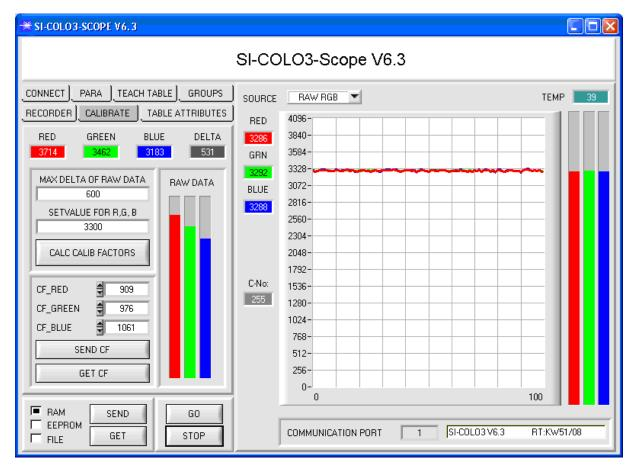
When the calibration factors have been calculated by the software on the user interface, they are automatically saved to the non-volatile EEPROM memory of the sensor. Calibration is then finished, work can then be continued in the main panel.
