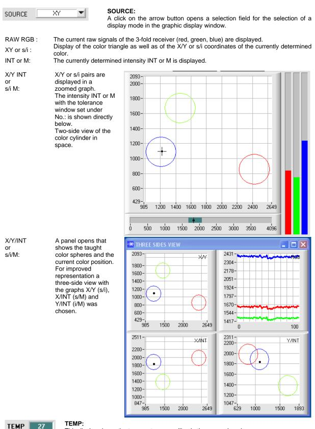
This display shows the temperature prevailing in the sensor housing. The display **DOES NOT** show degrees Centigrade or Fahrenheit
