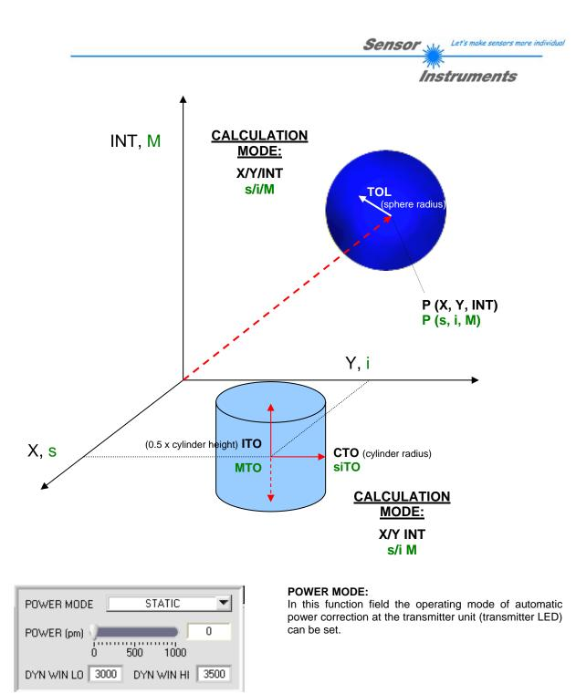
**STATIC:** The transmitter power is constantly kept at the value set with the POWER slider (recommended operation mode).
